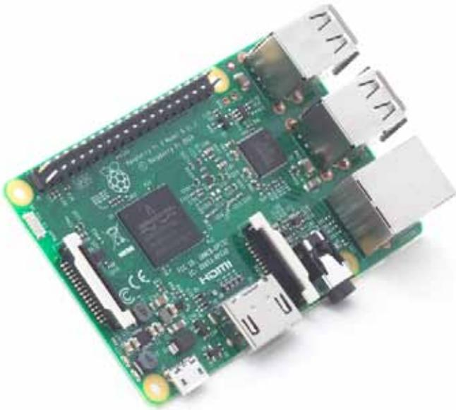
**Figure 3** – Raspberry Pi 3 (taken from [www.raspberrypi.org](http://www.raspberrypi.org))
